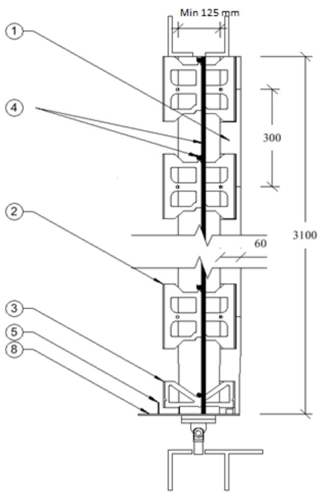
**Figure 2** Vertical section of the Polyfoam Polywall® ICF blocks (extracted from EWFA 2489001.1)
