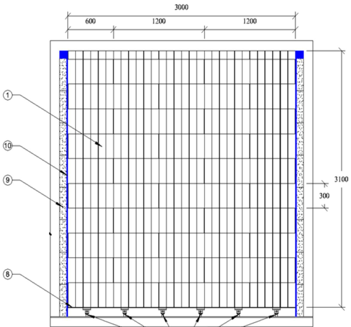
Figure 1 Face elevation of Polyfoam Polywall® ICF blocks (extracted from EWFA 2489001.1)
