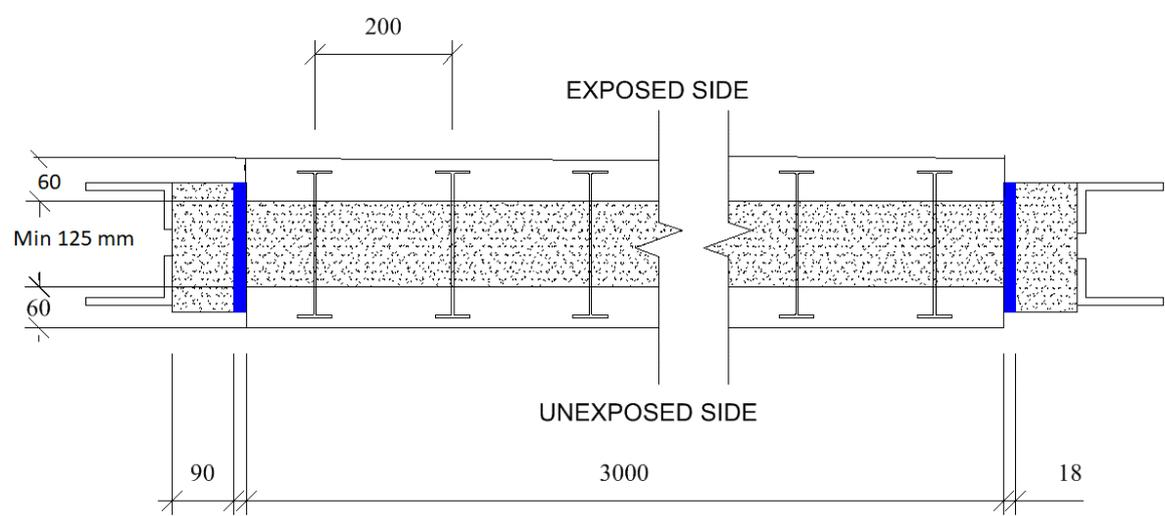
**Figure 3** Horizontal section of the Polyfoam Polywall® ICF blocks (extracted from EWFA 2489001.1)
