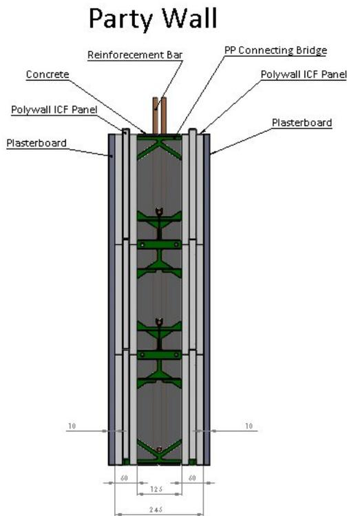
Figure 1: Structure of Polywall system
