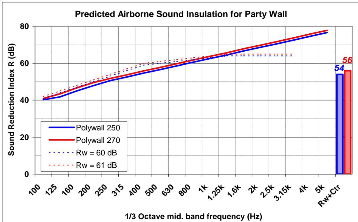
Figure 2: Prediction Sound Reduction Index for Polywall 250 & Polywall 270 systems (Party Wall)
